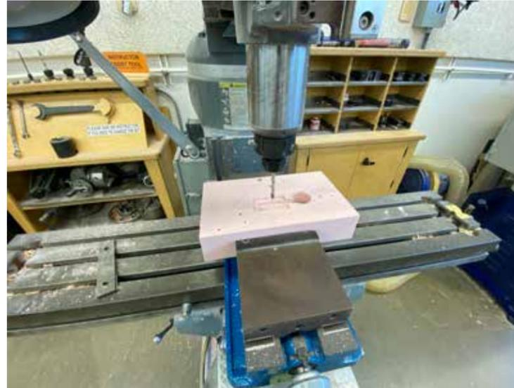
Milling the pocket for passive driver and the inner shared air space with the driver.
