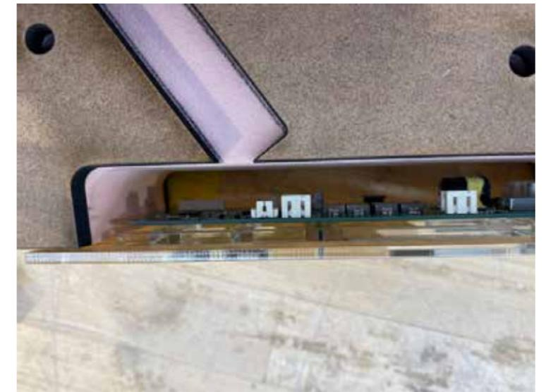
Laser PCB mounting panel to test the fit of the PCB pocket
