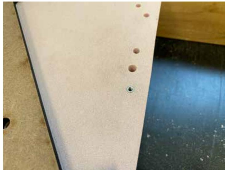
Testing the bit size for the screw inserts.
