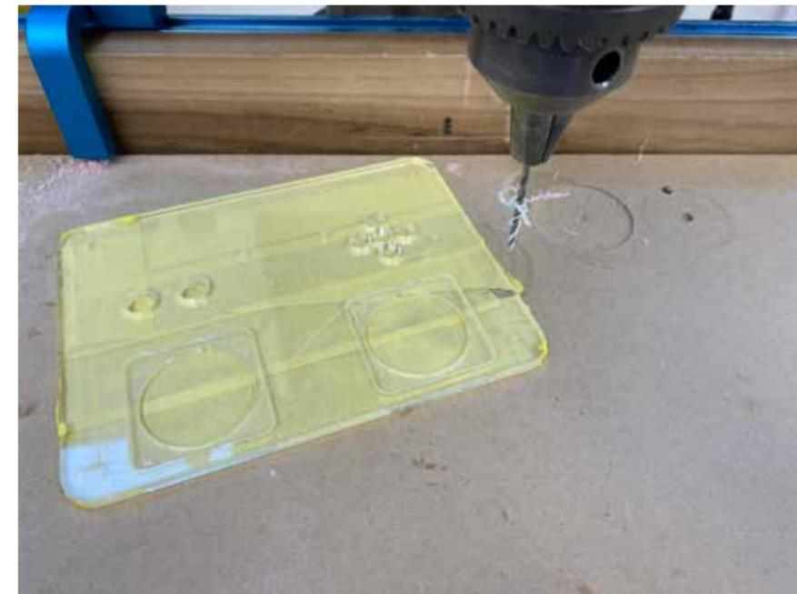
Drill and tap the screw hole on the front panel.
