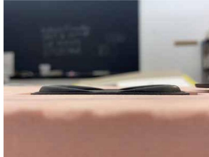
Making sure that the passive driver is tightly against the acrylic panel.
