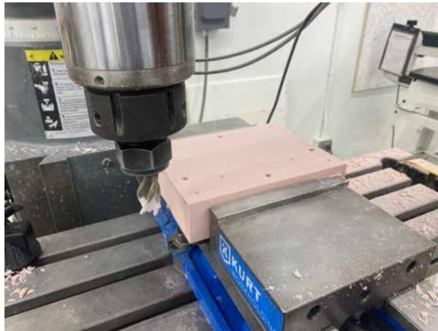
Mill the overall piece to the desired depth.
