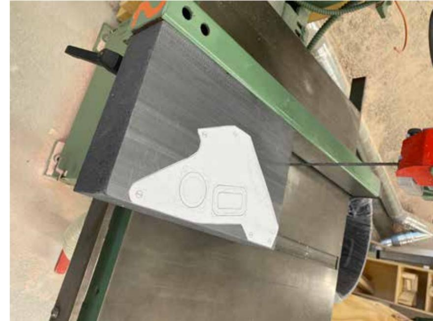
Cut the foam smaller but still maintain the rectangular shape to put on the mill
