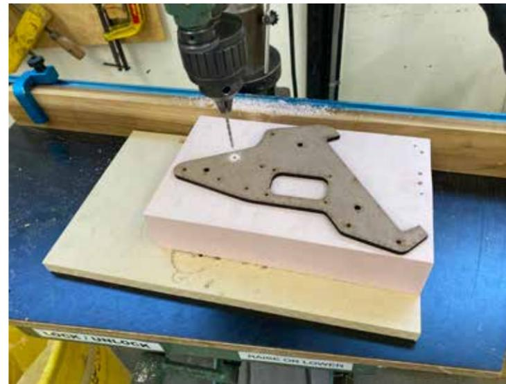
Drill all the thread insert holes based on the template.
