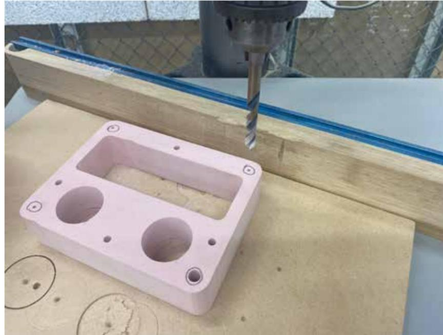
Drill the countersink hole for mounting the front panel.
