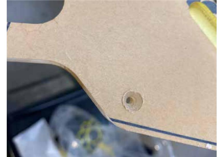
Counter sink all the screw hole on the acrylic panel.
